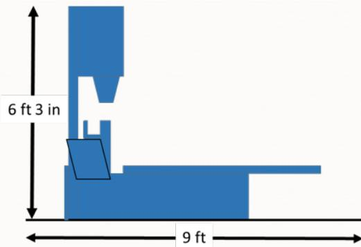
The Model SI-1 CBMT system occupies a footprint less than 24 sf. Powered from existing wall outlets, the complete and self-contained system can be operated from both sides to test both arms in floor space only 6' x 9'.
